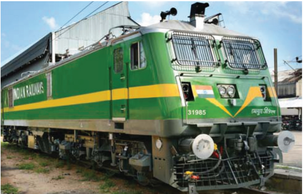
WAG 9 with IGBT based propulsion system
