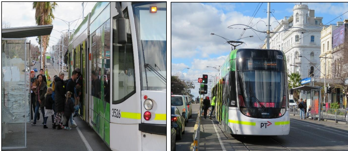
Low floor trams at non-DDA compliant stops
