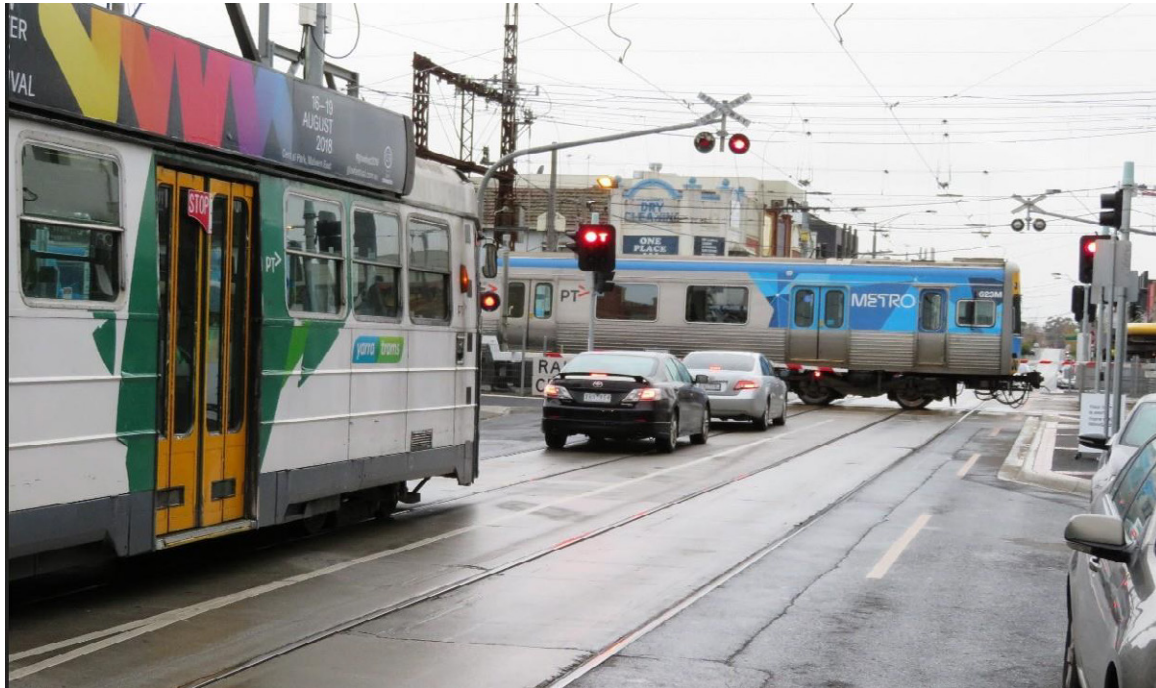
Train / Tram level crossing on the Frankston line at Glenhuntly Road, Glenhuntly
