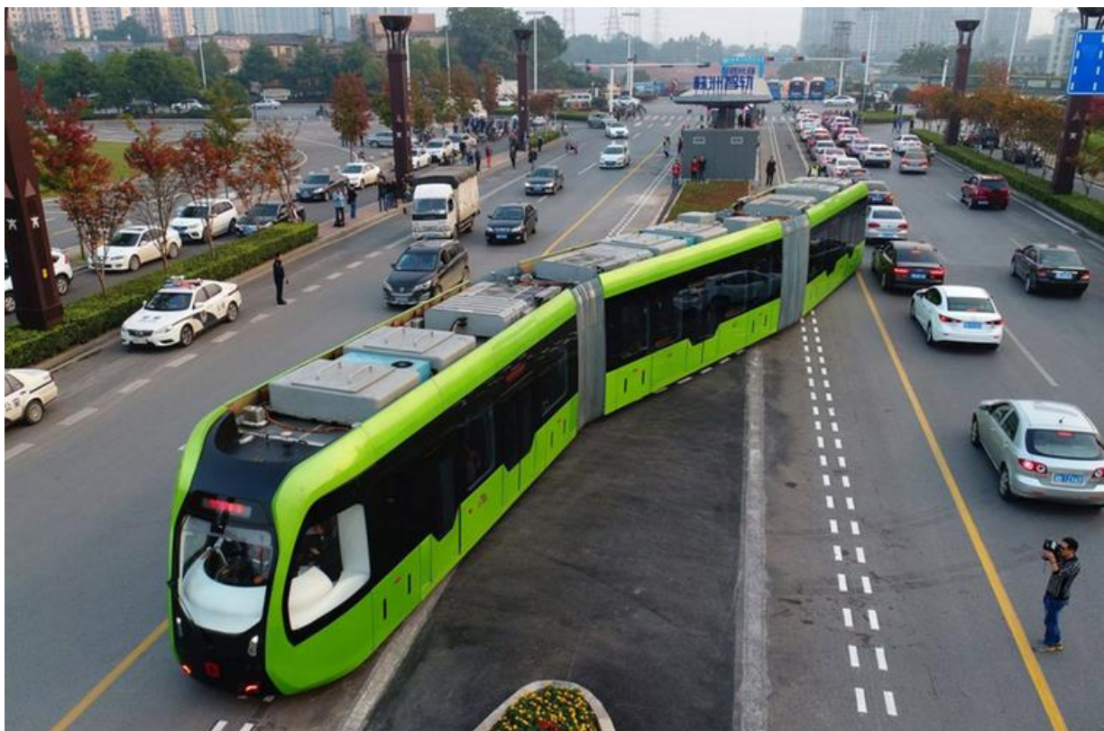
Experimental optically guided MCT vehicle, otherwise known as a "trackless tram" in Zhuzhou, Hunan Province, China
