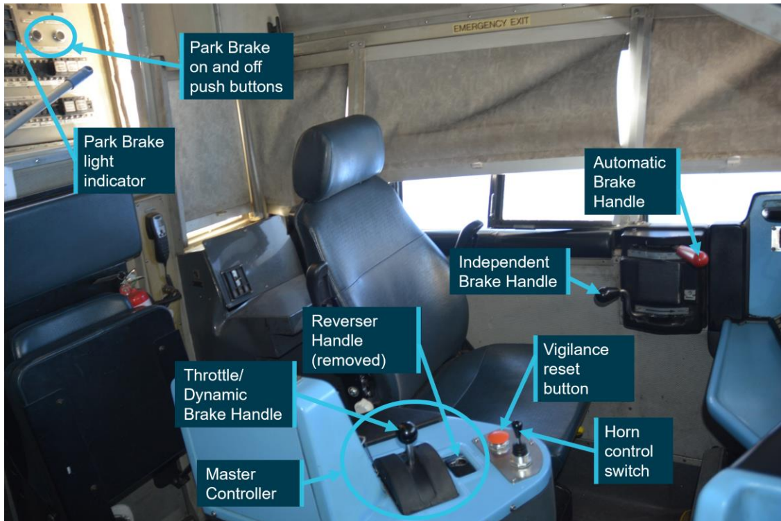
This figure shows the layout of the driver's controls Source: OTSI
