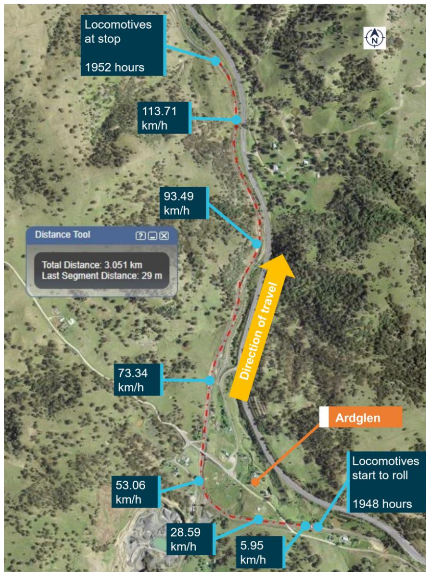
This figure shows the path of the runaway and the speed of the locomotives as they progressed from Ardglan towards Kankool. Source: SIX maps and ARTC trip report, modified by OTSI
